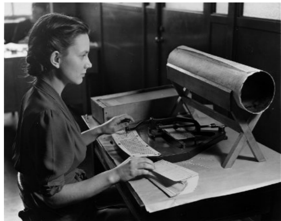
Fig. 2 Punched card and woman operating a keypunch. Source: Wikipedia, Punched card, https://en.wikipedia.org/wiki/Punched_card , access [07.12.2023].
